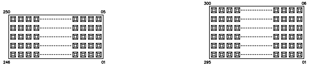
FIG. 2 POLARIZATION OPTION LOCATION INSERT PK-07 INTO SPECIFIED POSITION AND BREAK OFF TAB
